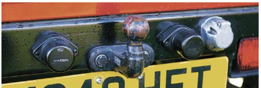
Rear cross member provides additional towball for carrying a bicycle rack
